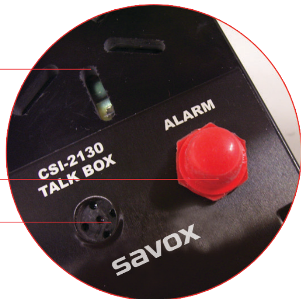
Plug Male Connector of Com Cable into Female Connector of the Talk Box
